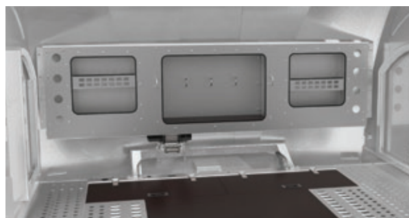
○ Store station with storage shelves and facility to carry 20 litre Jerry cans.
