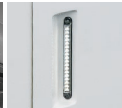
○ Additional reverse lights, these super bright side mounted LED reverse lights provide valuable extra visibility for close movement at night.
